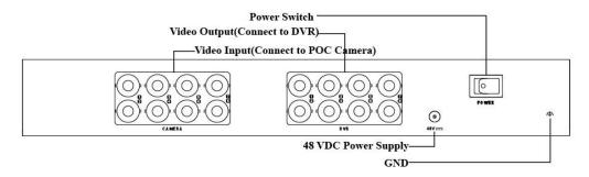
NOTE DS-1TP04I provides 4-ch video inputs and outputs.
